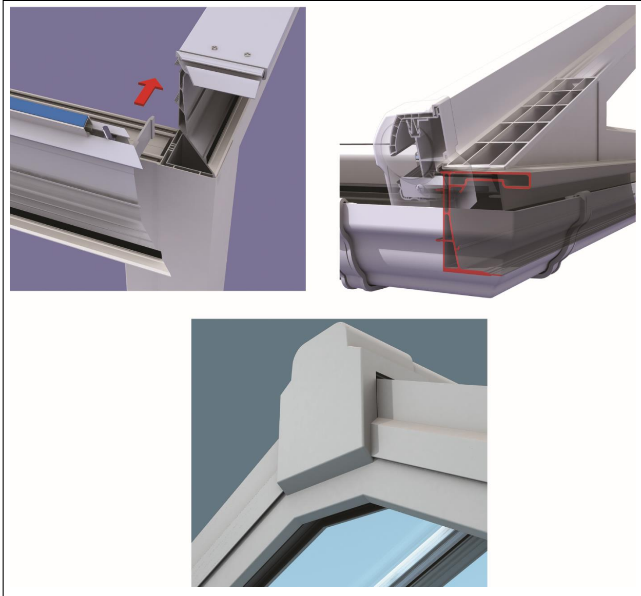
Figure 3 Gable support system
