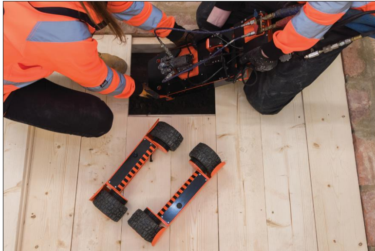
Figure 6 SprayBot installation through an air vent on the outside of the property
